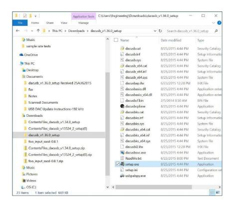
Open (unzip) the new USB DAC driver folder and install the new driver, using the "setup.exe" program, highlighted in the previous illustration.
